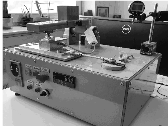
Figure 2. The pin-on-flat tribotester used in testing the friction coefficient
