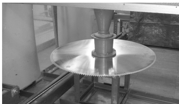
Fig. 3. Disc of cutting unit PI – 505 600 x 100 x 3,2
