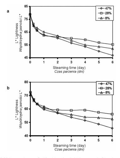
Fig. 6. Lightness change of white (a) and red (b) heartwood of beech at 110°C depending on the initial moisture content
