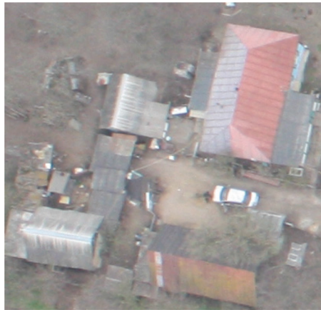
Figure 9. Contours blurred due to ISO increase.
