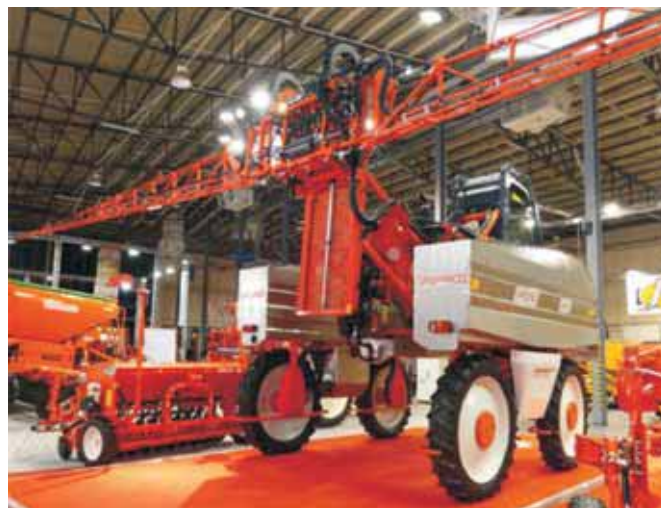
Rys. 2. Opryskiwacz samojezdny URAGANO (fot. S. Feder) Fig. 2. Self-Propelled Sprayer URAGANO (photo S. Feder)
