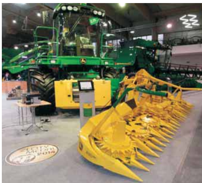
Rys. 3. Sieczkarnia John Deere serii 7080i z czujnikiem HarvestLab i procesorem KernelStar (fot. S. Feder) Fig. 3. Self-Propelled Forage Harvester John Deere 7080i series with HarvestLab sensor and KernelStar processor (photo S. Feder)
