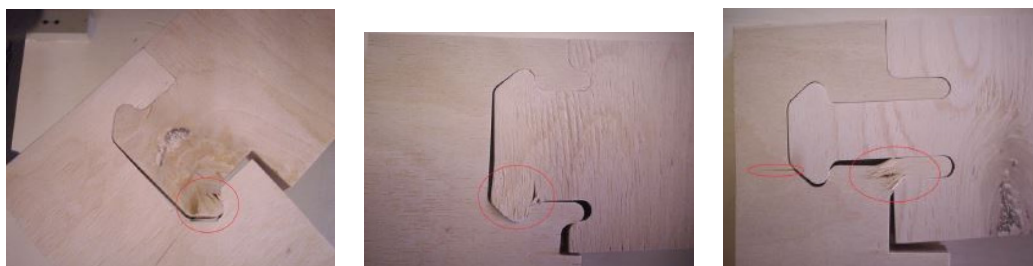
Fig. 6 Characteristic breach of joints under pressure load in the angular plane
