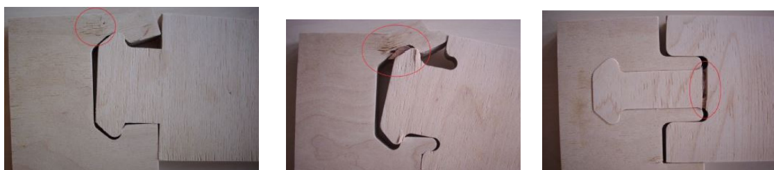
Fig. 4: Characteristic breach of joints under pressure load in the angular plane
