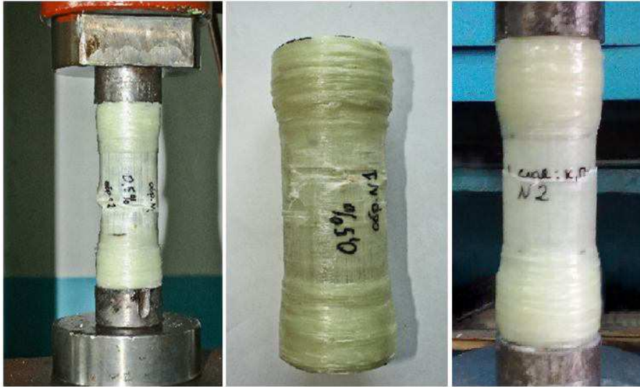
Fig. 1. TE sample in the testing adaptation and TE samples after the axial compressive loading
