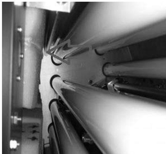
Figure 5. Mounting of the samples in a climate chamber
