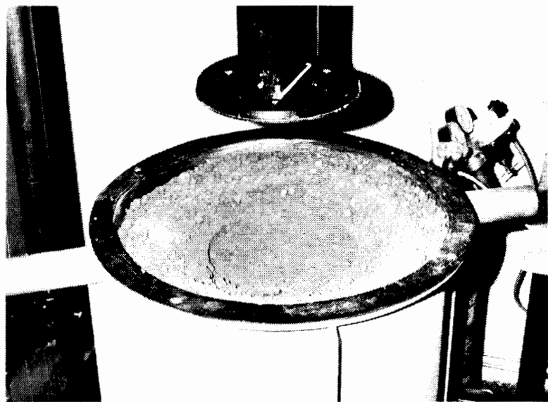
Fig. 2. Detail of the testing soil-bin filled with pre-compacted soil and of the compacting head holding the compacting plate size b
