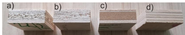
Figure 1. Tested sandwich panels with an inner layer made of: a) PB, b) OSB, c) MDF and d) glued PLY
