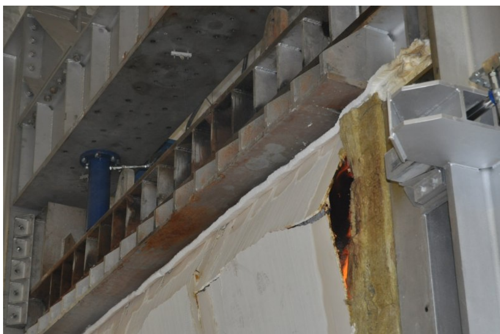
Photo 2 Loadbearing wall after achieved the criterion of loadbearing capacity (R)
