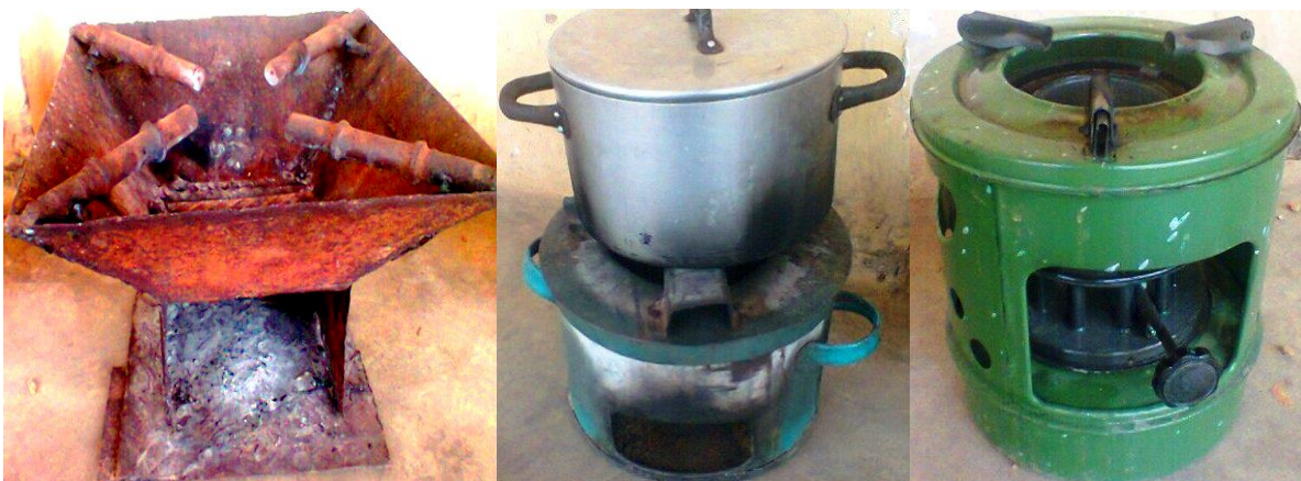
Figure 2. Test stoves: a) Charcoal, b) Sawdust / rice husk, c) kerosene.
