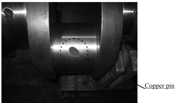
Fig. 2. A copper pin, installed on the damaged neck and polish flush
