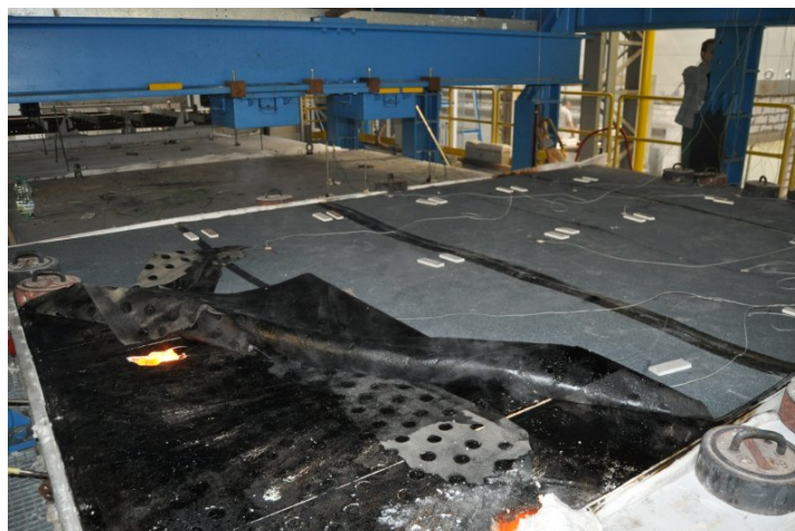
Fig. 3 Roof after finished test (top load removed and bitumen roofing membranes revealed)
