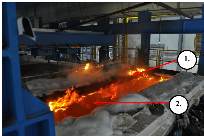
Fig. 4 Roof after finished test, where: 1 – wooden loadbearing beams, 2 – suspended weight. After the test (heating acc. to standard curve – time), the weights were removed from the roof (for safety reasons), and the bitumen roofing membranes were revealed. The bottom layer of the MgO boards were fell into furnace, the upper boards were fractured, locally holes were visible as shown in Fig. 3. During the following minutes (after the test) the bitumen roofing membranes were completely removed – the top boards also were fell into the furnace. Despite the complete damage of all roof layers, the revealed wooden members charring could still be observed – the suspended weights were fixed to the loadbearing beams and the beams themselves did not lose their loadbearing capacity. The actions described are shown in Fig. 4.
