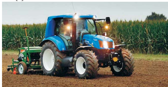
Rys. 5. Ciągnik New Holland T6.140 Metan Power [6] Fig. 5. Tractor New Holland T6.140 Metan Power [6]
