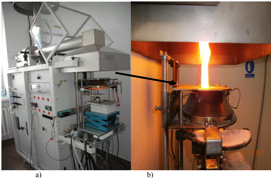
Fig.1. Experimental set-up of the cone calorimeter. a) Cone calorimeter, b) cone heater
