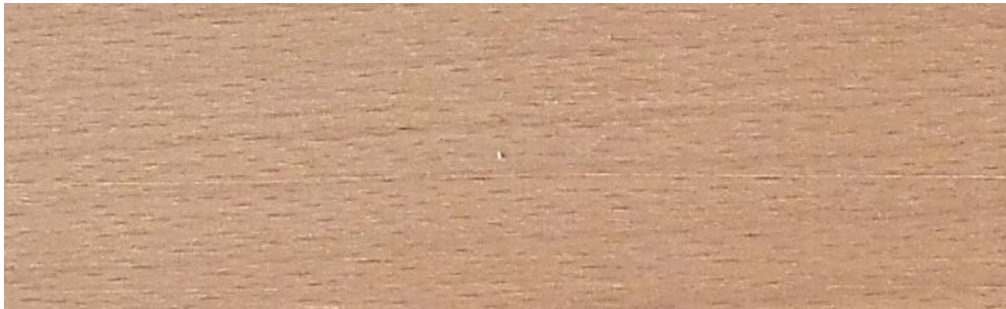
Figure 2. View of the beech wood after heat treatment.
