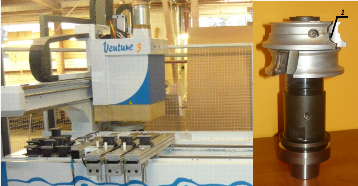
Fig. 1 A CNC Weeke Venture 3 woodworking machine and a ProfilCut cutterhead; 1 - knife used in tests
