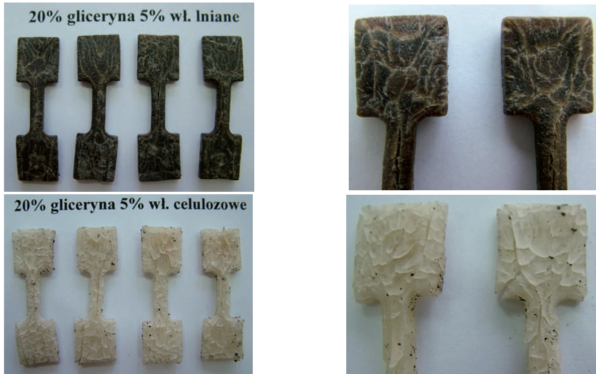
Fig. 10. The mouldings containing flax (a) and cellulose (b) fibers after 2 weeks storage time
