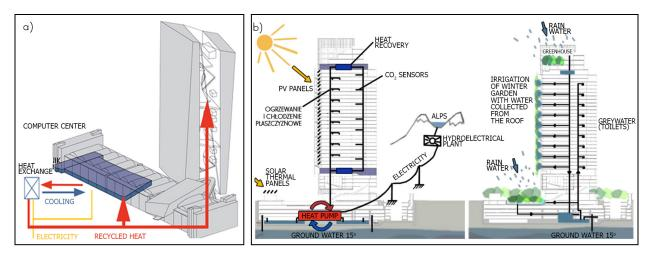
**Fig. 12.** High-tech solutions in high-rise buildings: a – ECB Tower, Frankfurt am Main, 2014: extracting heat from the computer centre; b – Grattacielo Intesa San Paolo, Turin, 2015: electricity from natural sources, HVAC system and installations – grey water and rainwater
