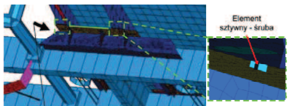
Fig. 6. The way of connecting front part of container with truck frame in exemplary garbage truck with the use of compression springs
