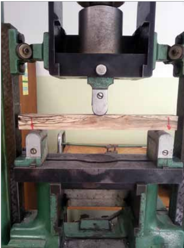
Figure 1. Static outline of sample support and load
