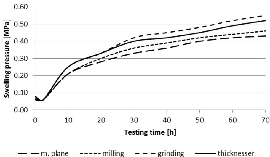
Figure 13. Swelling pressure depending on the different ways of forming the surfaces to be joined by a square joint at a preload of 0.06 MPa
