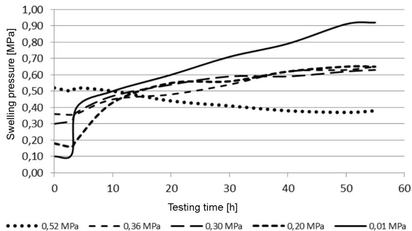
Figure 11. Swelling pressure depending on the size of the preload of the square joint of two oak wood surfaces
