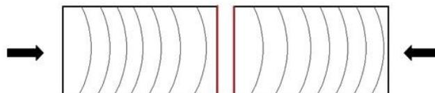
Figure 2: Arrangement of samples for testing the tightness of a square joint taking into account the direction of annual increments
