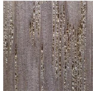
Figure 6. Contact surface after processing with abrasive paper grit 400, with visibly chipped grain
