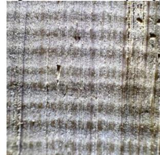
Figure 8. Contact surface formed using a thicknesser, characteristic deep wavy surface visible
