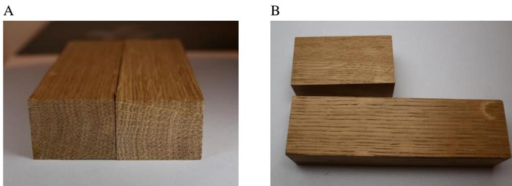
Figure 1: Radially cut oak samples 30 mm×40 mm (A) and 70 mm and 140 mm in length (B)
