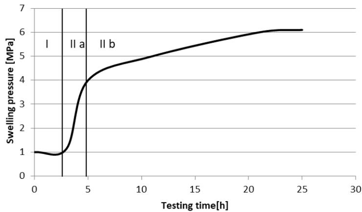
Figure 10. Characteristic areas of change in oak square joint swelling pressure at 0.1 MPa initial load
