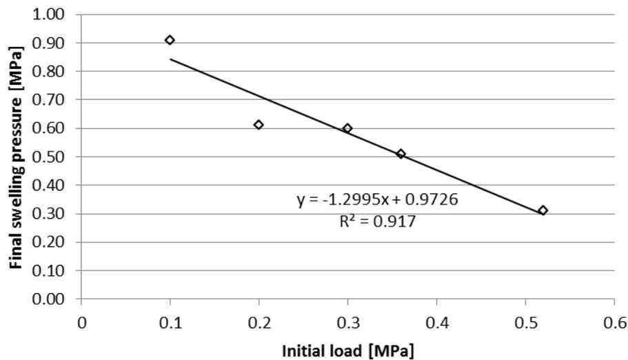
Figure 12. Size of swelling occurring between two surfaces connected by a square joint, at a preload of 0.1; 0.2; 0.3; 0.36 and 0.52 MPa after 55 hours of testing
