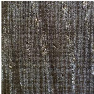
Figure 5. Contact surface after milling, with visible waves
