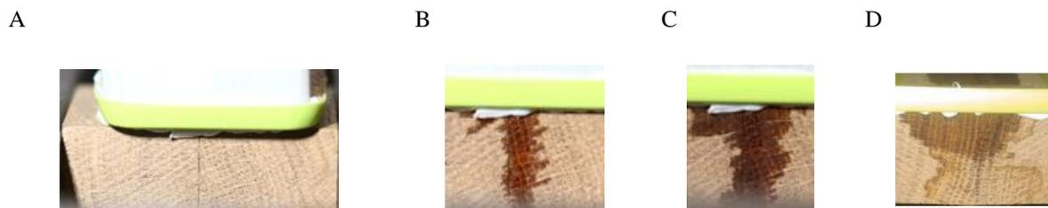
Figure 14. Moisture penetration through the joint. A – connected to the contact of the samples connected by a square joint prior to moistening, B – moisture penetration directly after pouring water into the vessel, C – after a few hours characteristic moistening of wood zones in the radial direction with moisture penetration through the joint, D – moment of joint tightening and drying of lower zones of the joined elements
