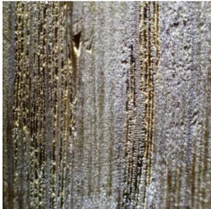
Figure 7. Contact surface after manual planing, with visible small waves
