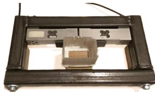
Figure 4. A measuring instrument with samples mounted in it, connected with a square joint, and a vessel with water insulated with silicone
