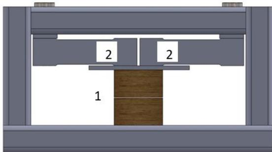
Figure 3. A diagram of a device for measuring swelling pressure and testing the tightness of a contact connection: 1-samples, 2-beam strain gauges
