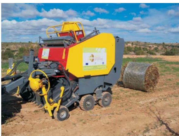
Rys. 2. Maszyna do zbierania i zwijania materiału drzewnego w sadach, w winnicach wg wynalazku PIMR Fig. 2. Machine for collecting and rolling up wood material in orchards, in vineyards according to the PIMR invention
