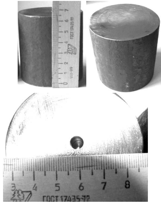
Fig. 1. The steel sample with an artificial reflector - drilling with a flat bottom: a - general view of the sample, b - a flat surface scanning with an ultrasound transducer, c - the flat surface of the sample with a flat bottom made by the drilling
