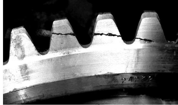
Fig. 5. Face plane of the locomotive gear with a visible defects
