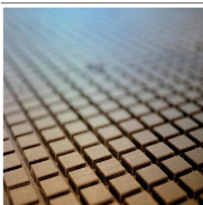
Fig. 4 The raster vacuum table used by "nesting"
