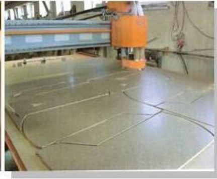
Fig. 2 Cutting board with nesting technology
