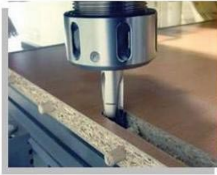
Fig. 1 Milling mortises in a board
