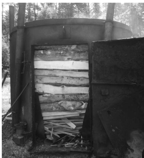
FIGURE 4. Retort fully loaded with sawmill wastes
