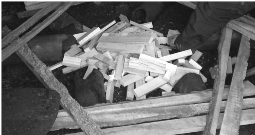
FIGURE 3. Floor with light-wood placed inside retort
