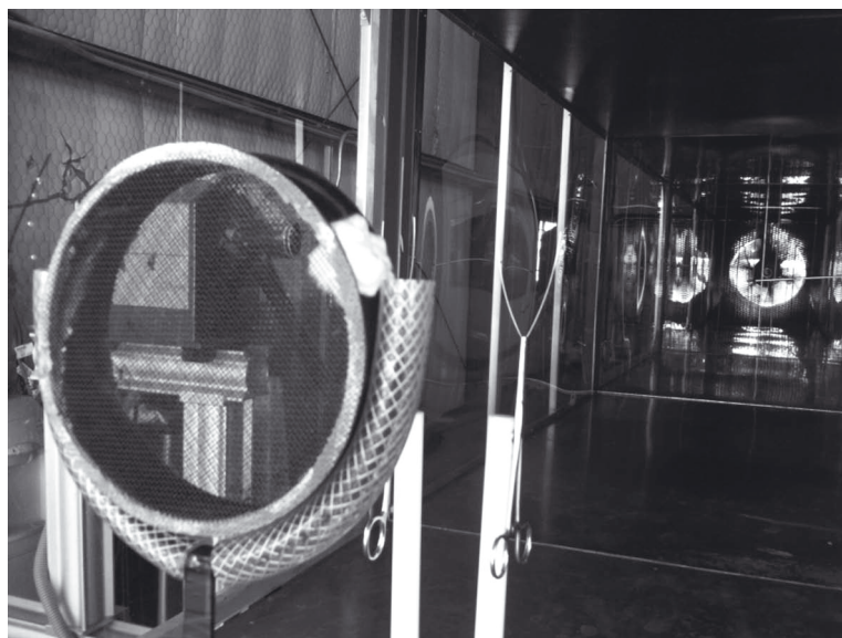
Fig. 2. Mosquito bioassay cage in position in the wind tunnel: the metal disk cage with volumetric line samplers up-wind of the cage
