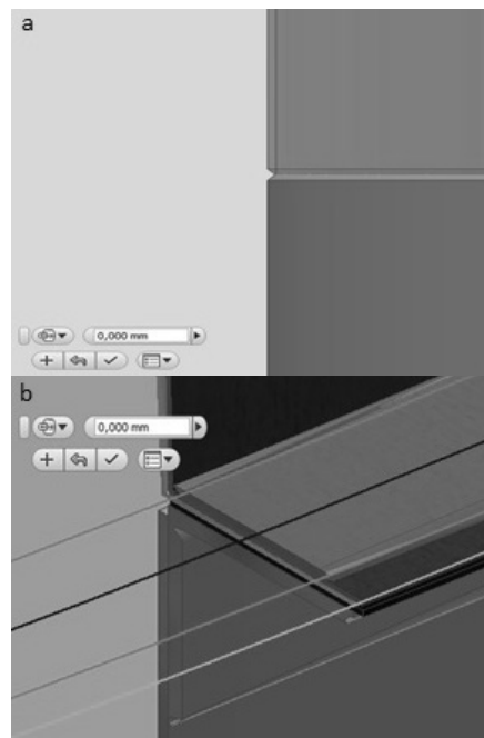
Fig. 10. Concentric connection of: a – tank's rings, b – ring pressing down on the membranes [own elaboration]
