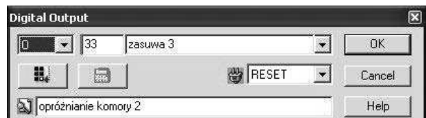
Fig. 3. Defining of the output signal for the control of the valve
