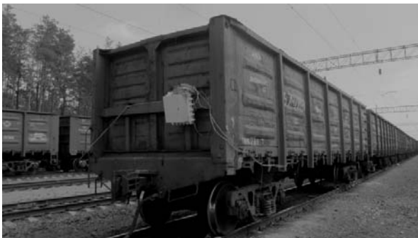
Fig. 2. Tests with the use of the mobile system in autonomous behavior of "black box"
