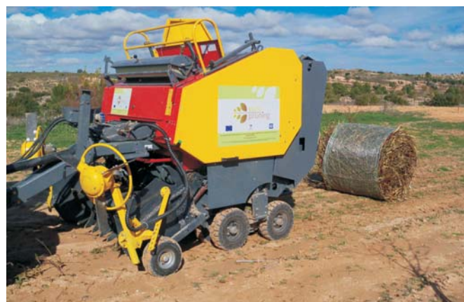
Rys. 7. Maszyna do zbierania i zwijania materiału drzewnego w sadach, w winnicach wg wynalazku PIMR Fig. 7. Machine for collecting and rolling up wood material in orchards and vineyards according to the PIMR invention
