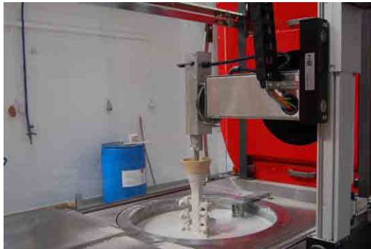
Fig. 3. Application of ceramic coating
