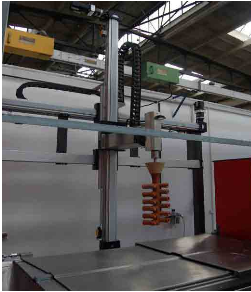
Fig. 2. Pattern set ready to make a ceramic mould
