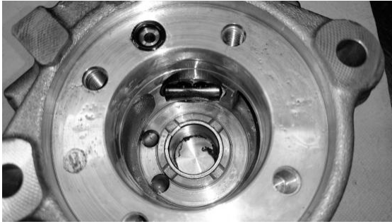
Fig. 5. A roller in the pump body in a faulty position
