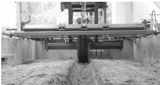
FIGURE 1. Measurement wheel and wheel-rut after driving along the channel
