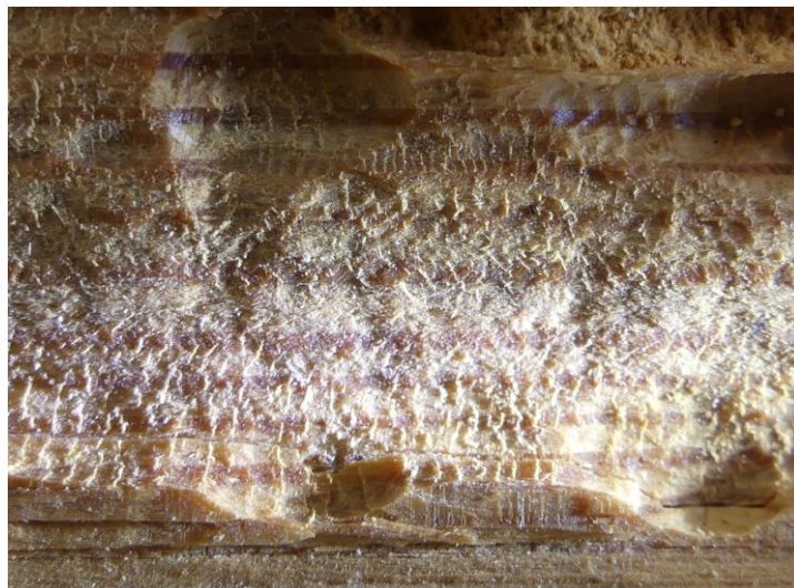
Figure 5. The surface texture of wood boring wall of old house borer ( Hylotrupes bajulus L.) in Scotch pine wood ( Pinus sylvestris L.)
