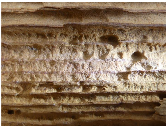
Figure 6. The surface texture of wood boring wall of Anobium punctatum L. in Scotch pine wood ( Pinus sylvestris L.)
