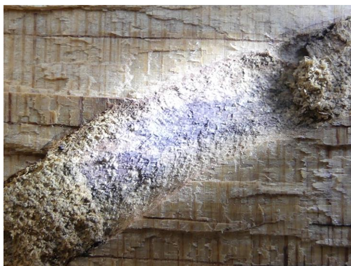
Figure 7. The surface texture of wood boring wall of Siricidae in Scotch pine wood ( Pinus sylvestris L.)
