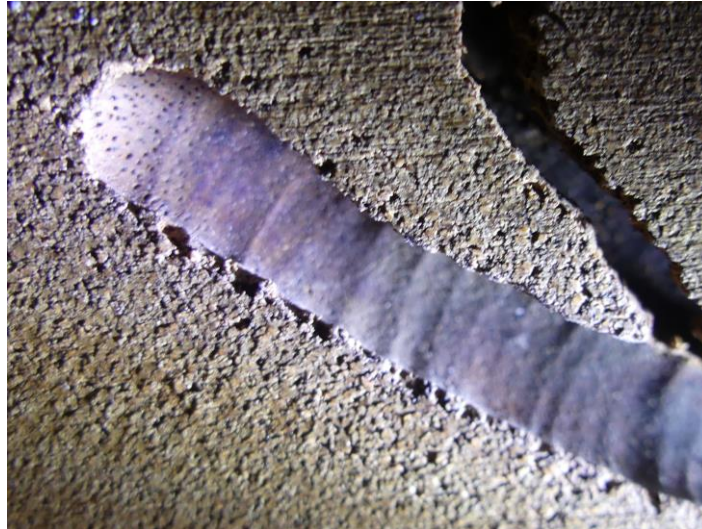
Figure 4. The surface texture of wood boring wall of Teredinidae in makore wood ( Tieghemella heckelii Pierre)
