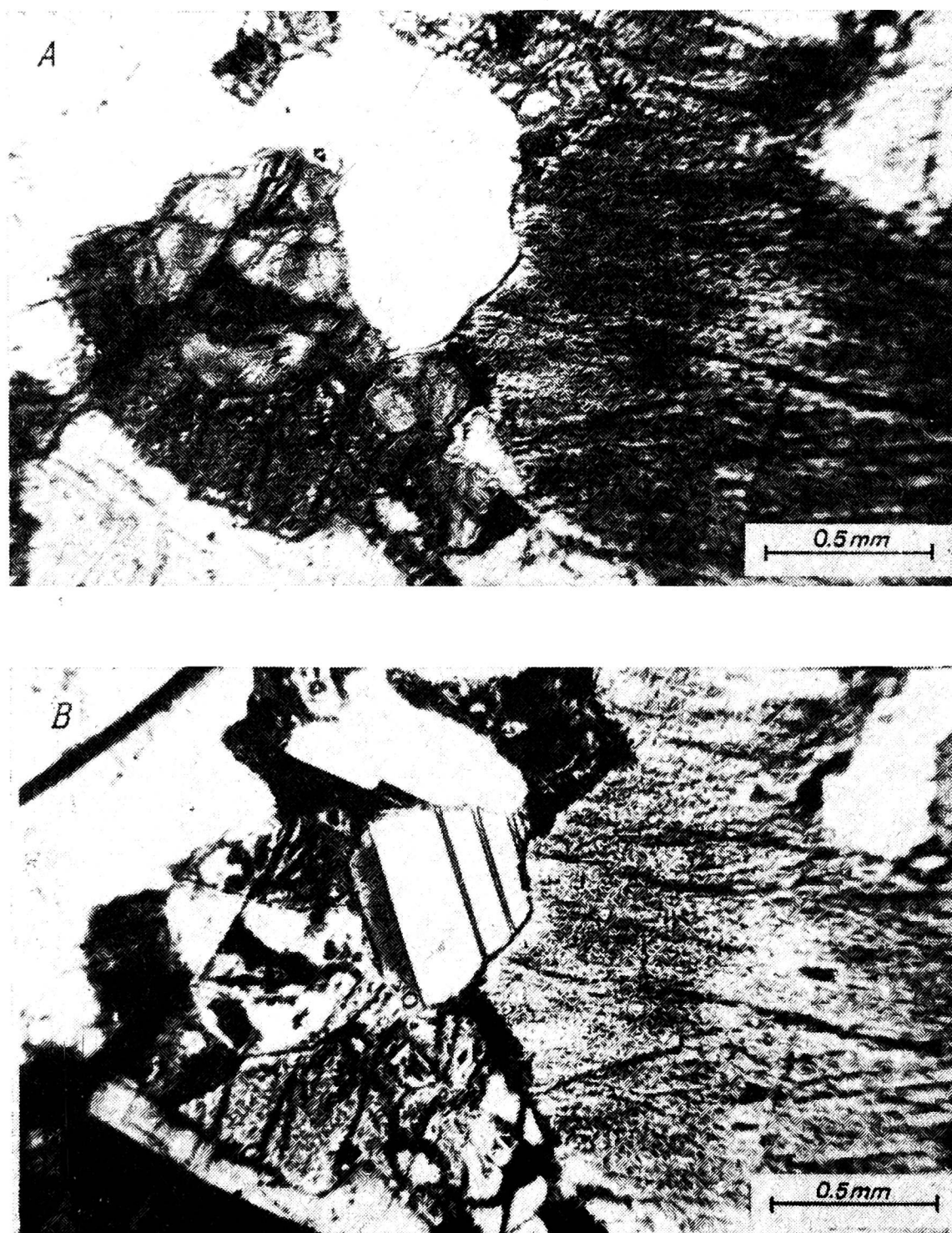
Fig. 3. Micromorphology of brown soil developed from olivine gabbro. Horizon C, depth 115-150 cm. Olivine gabbro as the parent rock. Main minerals show slight weathering. A — in plain light, B — under crossed polarizers.
