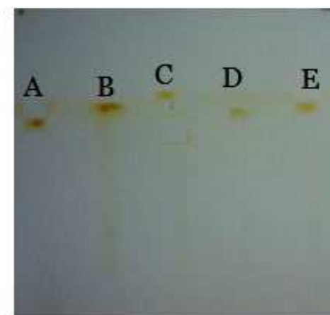
Figure 2: TLC sheet showing good retardation of crude sample with ethyl acetate and benzene (2:8).
