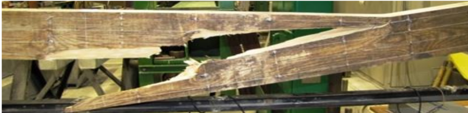
Fig. 8. Failure mode for the control beam URJF-1 (destruction of bases 6, 7, 8, 9, 10)
