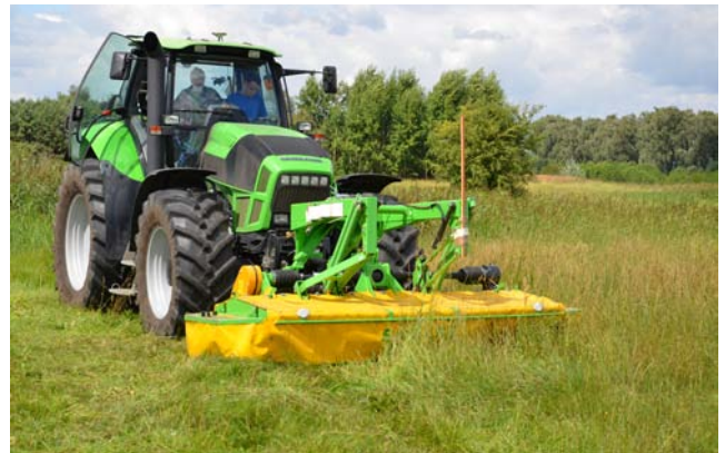
Figure 2. Tractor-mower set during field tests. Instantaneous absorbed powers for different body segments were computed from [11, 16]
