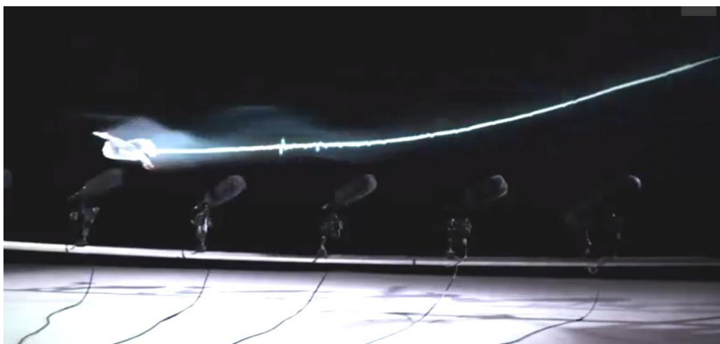
Figure. 6. Fly owls over microphones. no registered wing noise.
