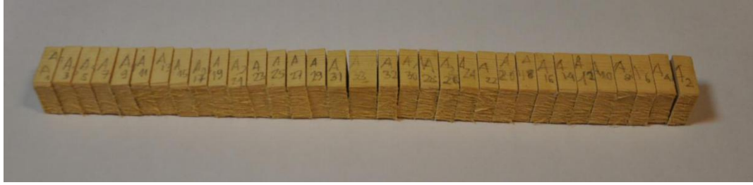
Figure 1. Example of a Norway spruce wood sample after alternate cutting off the beam ends
