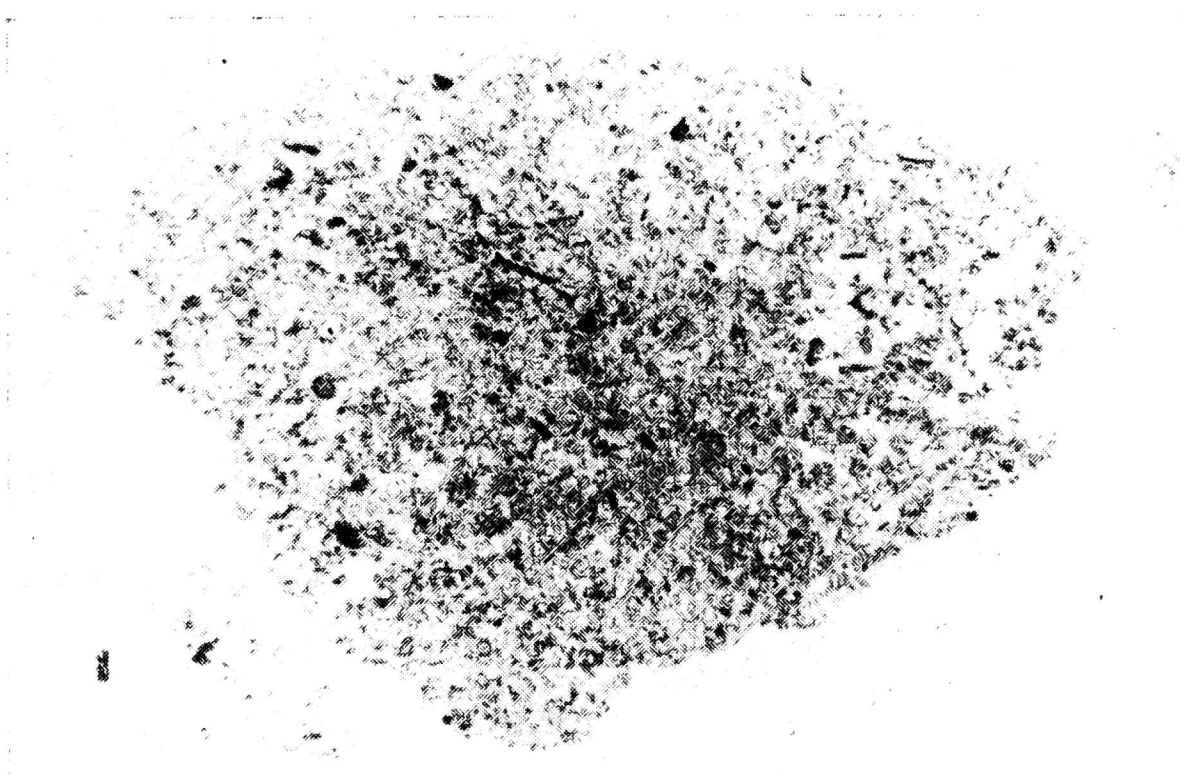
Fig. 10. Podzolic soil. Horizon A 1 . A fragment of aggregate 3-6 mm devoid of iron compounds, plain light. Magnif. about 20×.
