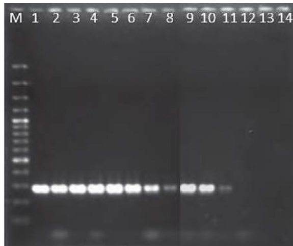
Fig. 5. Sensitivity of detection of Bacillus spp. strain 87 from tenfold dilutions of the bacterial DNA obtained by: Genomic Mini kit + BIO-PCR (lines 1-8) and by Boiling (lines 9-14): M – O'GeneRuler 100-3000bp (ThermoScientific, Life Science, Lithuania), 1 – 3x10 7 , 2 – 3x10 6 , 3 – 3x10 5 , 4 – 3x10 4 , 5 – 1.5x10 3 , 6 – 1.5x10 2 , 7 – 1.5x10 1 , 8 – 1.5x10 0 , 9 – 1.5x10 7 , 10 – 1.5x10 6 , 11 – 1.5x10 5 , 12 – 1.5x10 4 , 13 – 1.5x10 3 , 14 – 1.5x10 2
