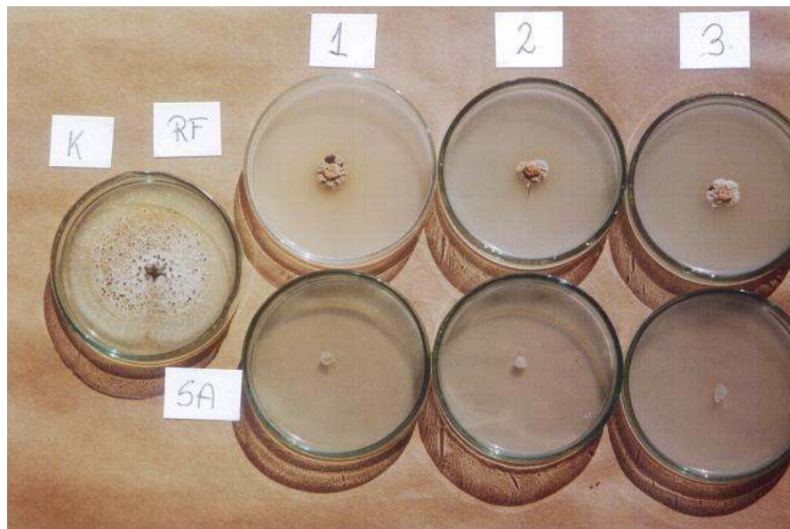
Photo 3. An effect of fungicides on linear growth Rhizosphaera kalkhoffii (K – control; RF, SA –Rovral Flo 255 SC and Sportak Alpha 380 EC, respectively; 1 – concentration 0.075% for Rovral Flo i 0.025% for Sportak Alpha; 2 – concentration 0.15% for Rovral Flo i 0.05% for Sportak Alpha; 3 – concentration 0.225% for Rovral Flo and 0.075% for Sportak Alpha)
