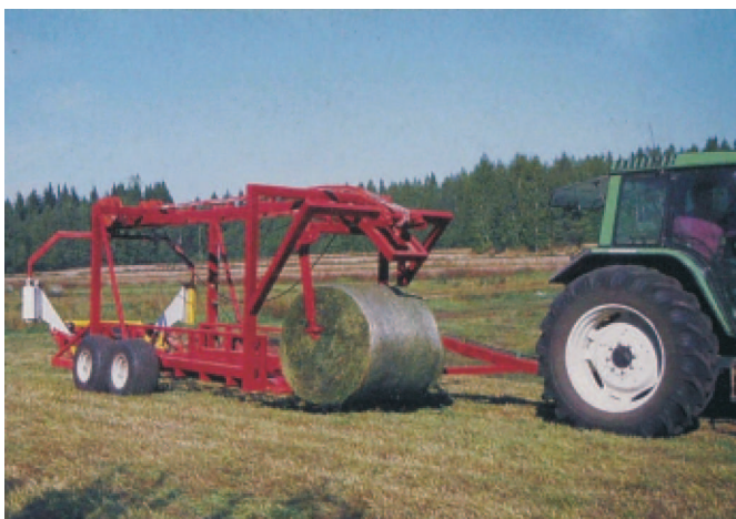
Rys. 7. Owijarka NHK 600 3D Stargate Fig. 7. The NHK 600 3D Stargate round bale wrapper
