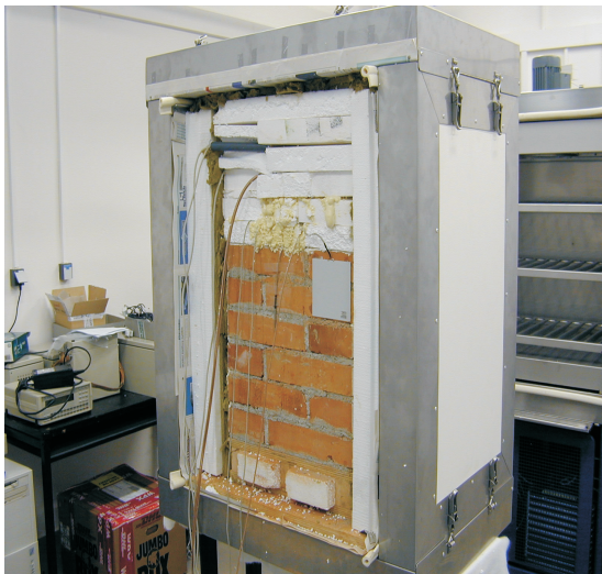
Fig. 3. Specimen insulation in the connecting tunnel (exterior surface).
