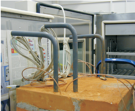
Fig. 2. Placing of TDR sensors into the tested structure.
