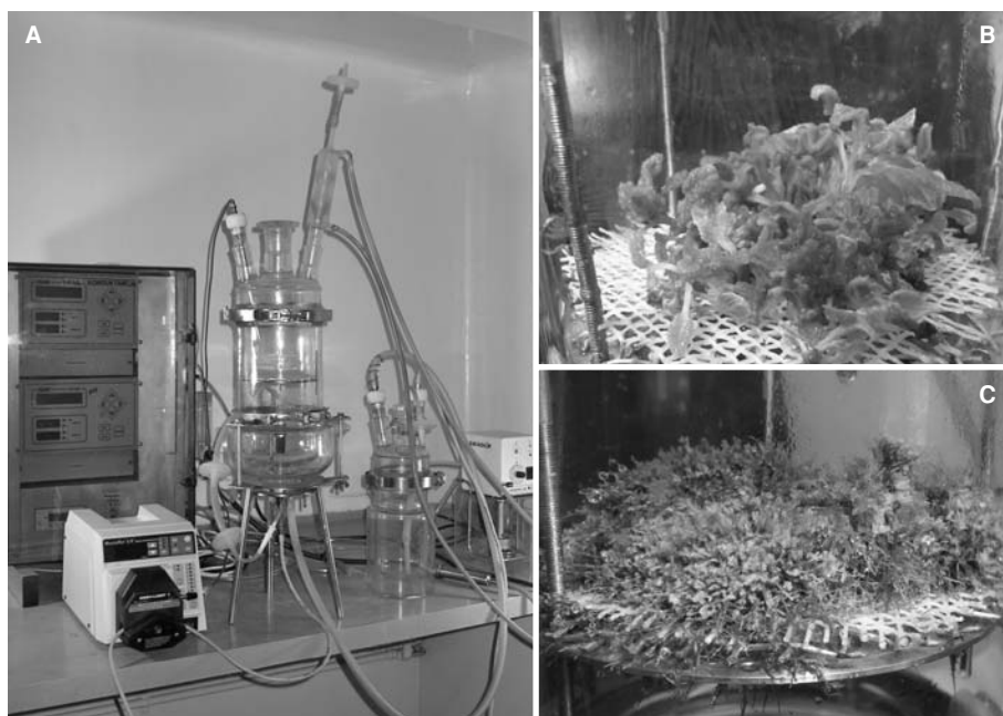
Fig. 1. Nutrient sprinkle bioreactor tested in the experiments: set-up for the design (A); biomass of Salvia officinalis shoots (B) and hairy roots (C) harvested after 21 and 40 days of inoculation, respectively.
