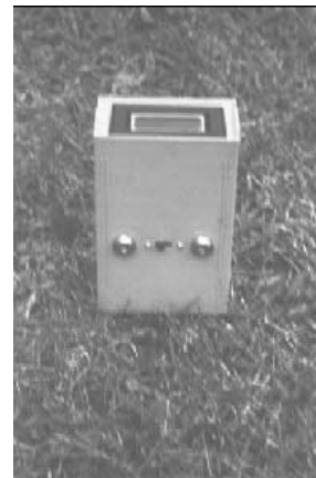
Fig. 10. The prototype based on the model of the impedance of soil probe.
