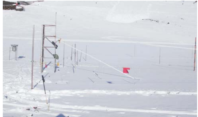
Fig. 3. The cable sensor system at Weissfluhjoch Davos (2550 m): the electronic devices in the shelter (left) and the test field with sloping cable sensor (right).
